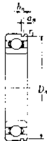
With Snap Ring Groove 62N
